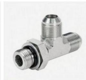
P/N:AJJO-OG JIC male 74° cone/sae o-ring run tee
