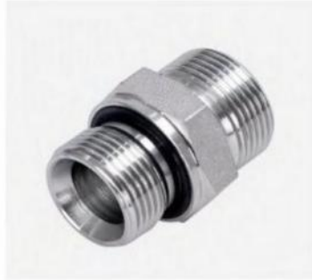
P/N:1CB-WD Metric male 24° cone L.T/BSP male with captive seal
