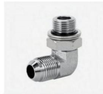
P/N:1JG9-OG 90°elbow JIC male 74° cone /sae o-ring boss l-series
