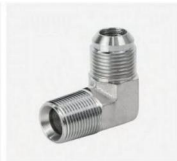
P/N:1JT9 90°elbow JIC male 74° cone/BSPT male
