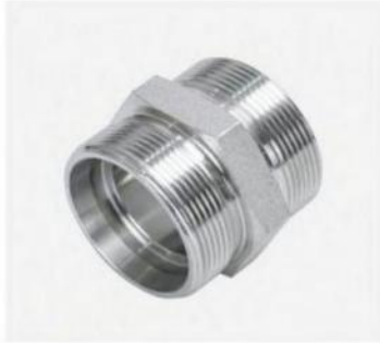
P/N:1C Metric male 24° cone L.T/BSP male with captive seal
