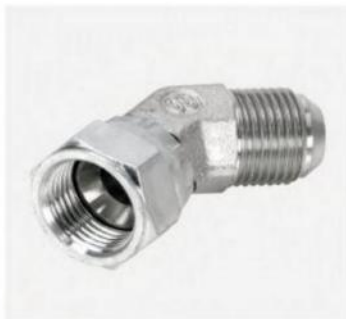
P/N:2J4 45° JIC female 74° cone/JIC male 74° cone
