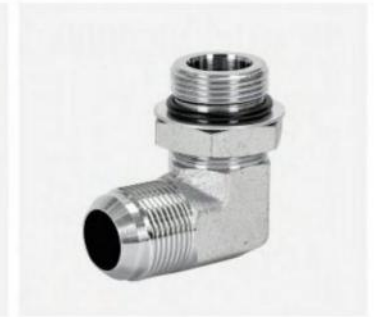
P/N:1JO9 90°elbow JIC male 74° cone /sae o-ring
