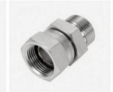
P/N:2B BSP male double use for 60° seat or bonded seal/BSP female 60° cone
