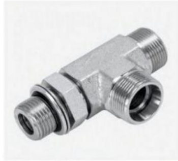
P/N:ACCG-OG BSP thread adjustable stud end with o-ring sealing run tee
