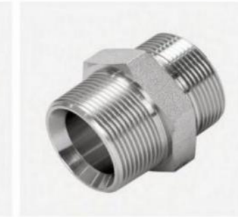
P/N:1BN/1BT BSP male double use for 60° seat or bonded seal/BSPT(NPT) male
