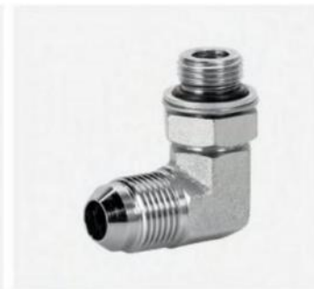
P/N:1JH9-OG 90°elbow JIC male 74° cone /metric adjustable stud end l-series
