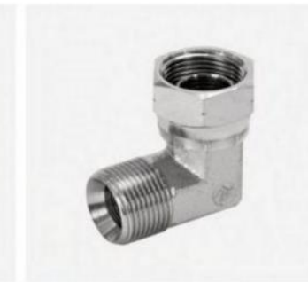
P/N:2B9 90° BSP male double use for 60° seat or bonded seal/BSP female 60° cone
