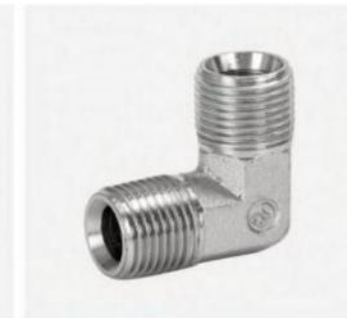
P/N:1BN9/1BT9 90° elbow BSP male 60° seat/NPT male
