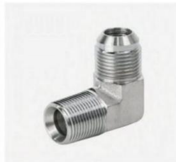
P/N:1JN9 90°elbow JIC male 74° cone/NPT male
