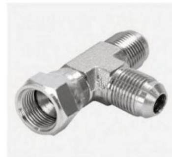
P/N:CJ JIC male 74° cone/JIC female 74° seat run tee
