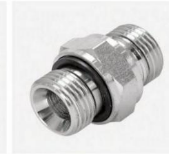
P/N:1B-WD BSP male double use for 60° seat or bonded seal/BSP male captive seal
