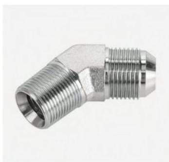
P/N:1JN4 45° elbow JIC male 74° cone/NPT male
